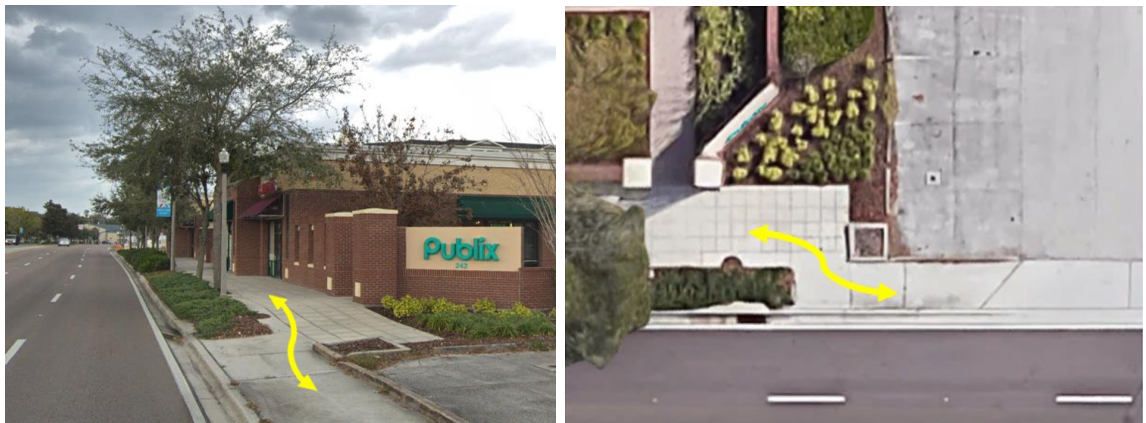
Figure XIV - 7. Connecting Existing and New Sidewalks
